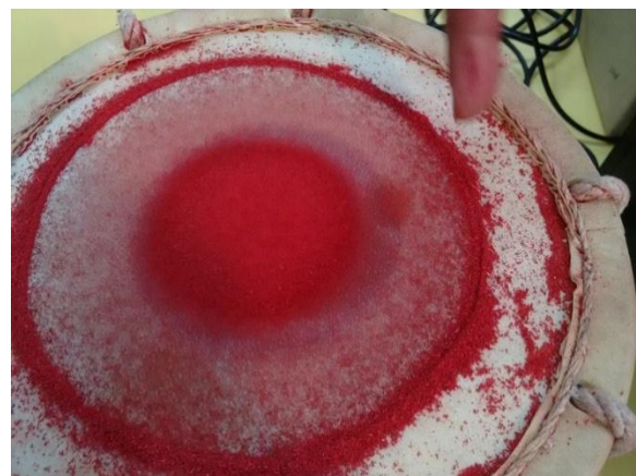
Fig. 5. Mode (0, 2): Stained sawdust accumulating around boundaries
