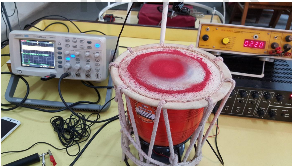
Fig. 9(b). Photograph of the setup for concurrent modal and spectral analysis by indirect excitation
